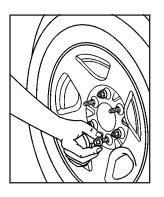
After mounting the spare, put the wheel nuts back on with the rounded end of the nuts toward the wheel. Tighten each wheel nut by hand. Then use the wheel wrench until the wheel is held against the hub.
